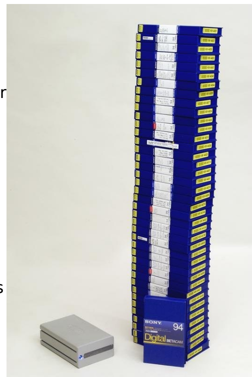
Forty Betacam tapes are needed for the data that fits on a 1TB hard drive
