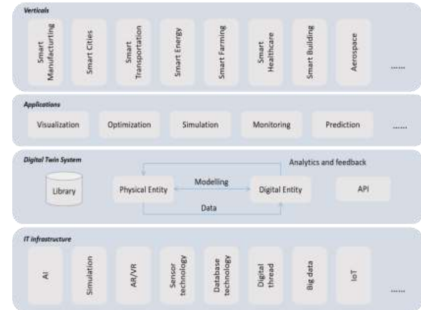
PWI JTC1-SC41-5 Digital Twin – Reference Architecture
