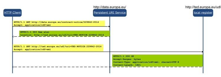
Figure 3: Sequence diagram: external HTTP redirection (forwarding)
